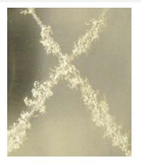
Both samples were scribed with an X and exposed to NSS for 23 hours and were placed in humidity cabinets set @40°C and 80% RH for 6 weeks
