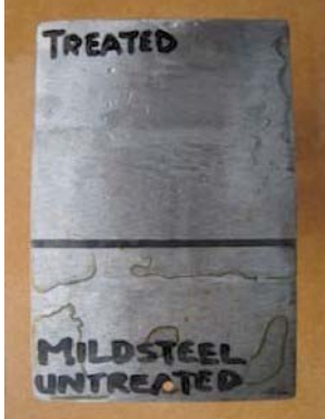
Mild steel after 1 day, showing heavy electrolysis starting to occur on the untreated surface.
