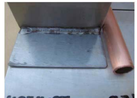
Treated side of the assembly after 10 days is showing no corrosion or electrolysis.
