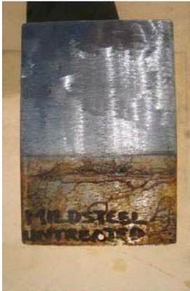
Mild steel after 1 month, the rust and electrolysis is much heavier and the untreated side is showing no effect.
