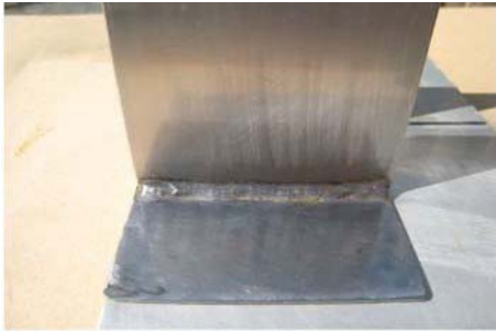
Treated side after 1 month is showing no corrosion or electrolysis.
