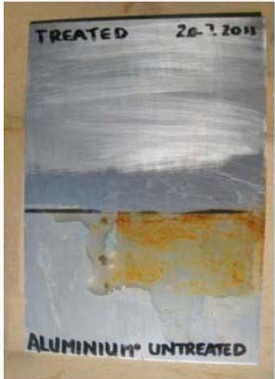
Aluminum after 1 month showing rust,. The rust is truly setting in. Where the copper tube is sitting, the aluminum is being eaten away in 3 spots in particular due to electrolysis.
