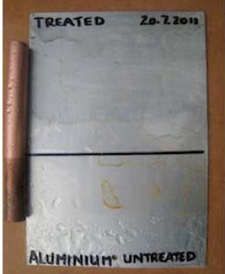
Aluminum after 1 day showing rust, and beginnings of electrolysis occurring, on the untreated half of the aluminum.
