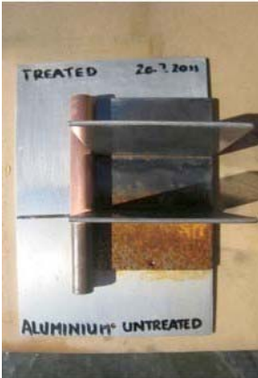
Aluminum after 1 month showing rust,. The rust is truly setting in. Where the copper tube is sitting, the aluminum is being eaten away in 3 spots in particular due to electrolysis.
